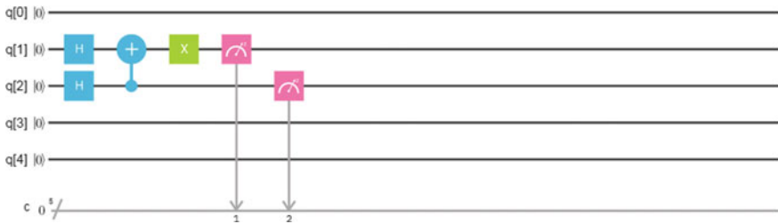
Fig. 2.26 The corresponding quantum circuit of the program in Listing 2.9
