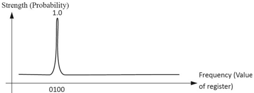
Fig. 4.16 After the inverse quantum Fourier transform of sampling sixteen points in Fig. 4.12, the frequency of signal is the measured outcome of the quantum register with four quantum bits and its strength is the possibility of reading out the outcome
