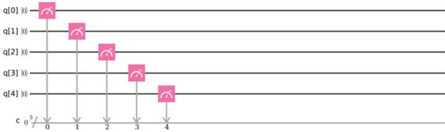
Fig. 1.2 The quantum circuit of declaring and measuring five quantum bits
