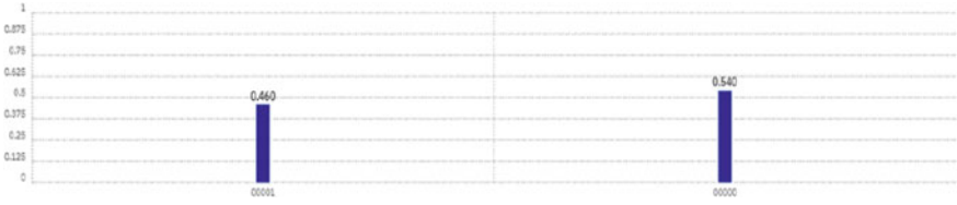
Fig. 1.30 After the measurement to the program in Listing 1.10 is completed, we obtain the answer 00001 with the probability 0.460 or the answer 00000 with the probability 0.540
