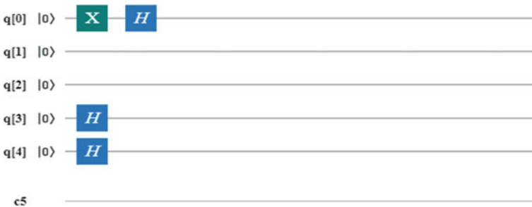
Fig. 3.2 The quantum circuit of constructing solution space to an instance of the satisfiability problem with F(x_1, x_2) = x_1 \wedge x_2
