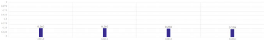
Fig. 2.24 After the measurement to the program in Listing 2.8 is completed, we obtain the answer 00010 with the probability 0.260 or the answer 00110 with the probability 0.260 or the answer 00100 with the probability 0.250 or the answer 00000 with the probability 0.230
