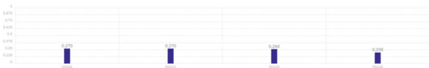
Fig. 2.21 After the measurement to the program in Listing 2.7 is completed, we obtain the answer 00001 with the probability 0.270 or the answer 00010 with the probability 0.270 or the answer 00100 with the probability 0.260 or the answer 00110 with the probability 0.200
