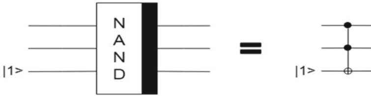
Fig. 2.13 The quantum circuit of implementing NAND operation of a classical bit
