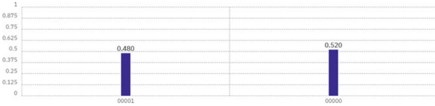
Fig. 1.24 After the measurement to the program in Listing 1.8 is completed, we obtain the answer 00001 with the probability 0.480 or the answer 00000 with the probability 0.520
