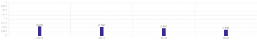
Fig. 2.12 After the measurement to the program in Listing 2.4 is completed, we obtain the answer 00010 with the probability 0.290 or the answer 00111 with the probability 0.280 or the answer 00100 with the probability 0.240 or the answer 00000 with the probability 0.190
